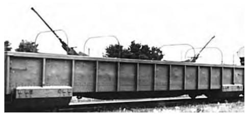
**More Problems...**To add to the problems the rail bed was in need of up grading. Ties were rotting and some spikes were so loose they could be removed by hand. The resulting vibration necessitated lowering the speed to 10 to 15 mph. The vibrations played havoc with the search lights and gun mountings which were attached solidly to the floors of the rail cars. The cars had to be sent to Vancouver for upgrades and returned in November. Changes
