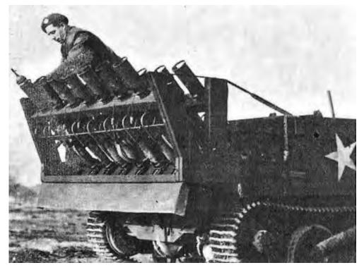
Improvised by the Canadians in 1944, this consisted of 14 PIAT projectors mounted on a frame at the rear of the carrier in two series of seven. Each row could be fired simultaneously by means of a mechanical contrivance of steel rods attached to the firing triggers. A few vehicles so fitted were used in Europe in 1944-45.
