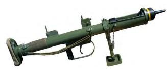
es. The most common misconception about the PIAT is that the bomb was propelled by the weapon's powerful mainspring. In reality, it was launched by a small but potent cartridge located in the base of the projectile using the spigot mortar principal. The spring's main task was to soak up the formidable recoil of the weapon so that it could be fired from a soldier's shoulder and to propel the PIAT's spigot forward to detonate and launch the bomb.
